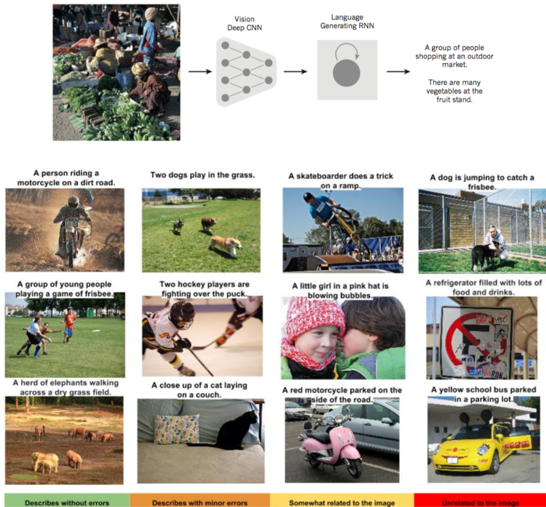
Figure 3. From image to text. It generates complete sentences in natural language extracted by a deep convolution neural network (CNN) an input image from a test image, with the RNN trained to ‘translate’ high-level representations of images into captions (top). A selection of evaluation results grouped by human rating (bottom).
